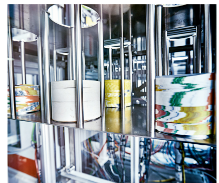
Fig. 1. In each processing step, the IML system takes six labels at a time from a magazine and places them into the open mold of the injection molding machine © Beckhoff Automation
